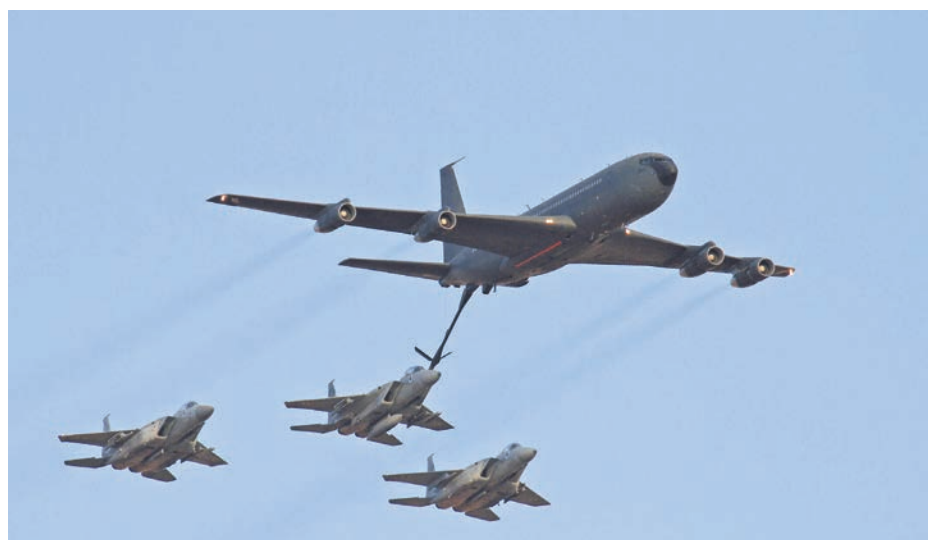
An Israeli Air Force Boeing 707 tanker aircraft fuels an IAF F-15 fighter jet, June 28 2011. Credit: Ofer Zidon/Flash90
